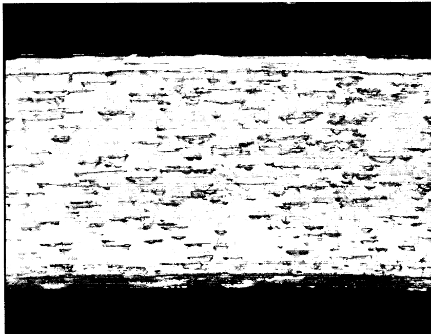
Fig. VII-21. Photomicrograph of a cross section of a high-Ag modification to an Au-1 wt% Ag proprietary electroplate on a Solacel.
